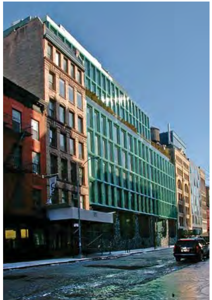
A street wall of five floors with upper floors stepped back (40 Bond Street in Manhattan designed by Herzog & de Meuron). 7
