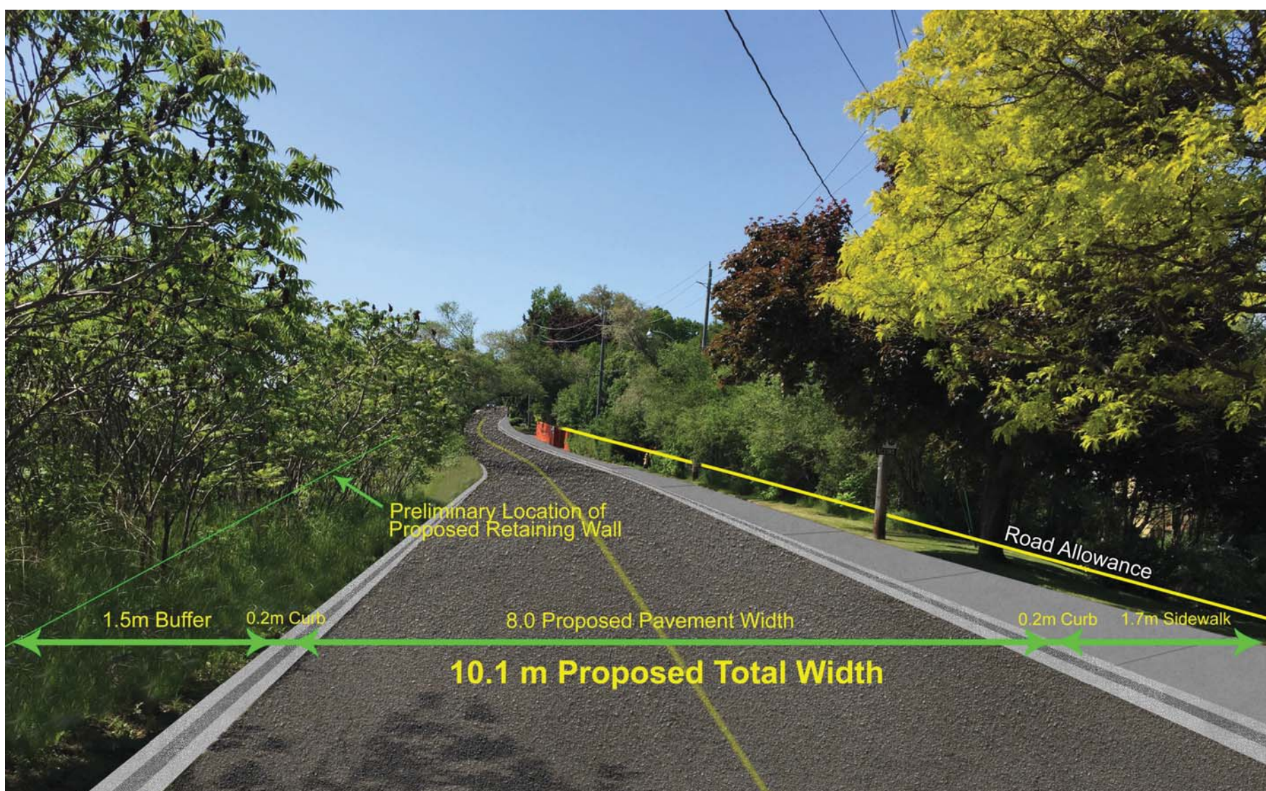
Proposed Road Cross Section
