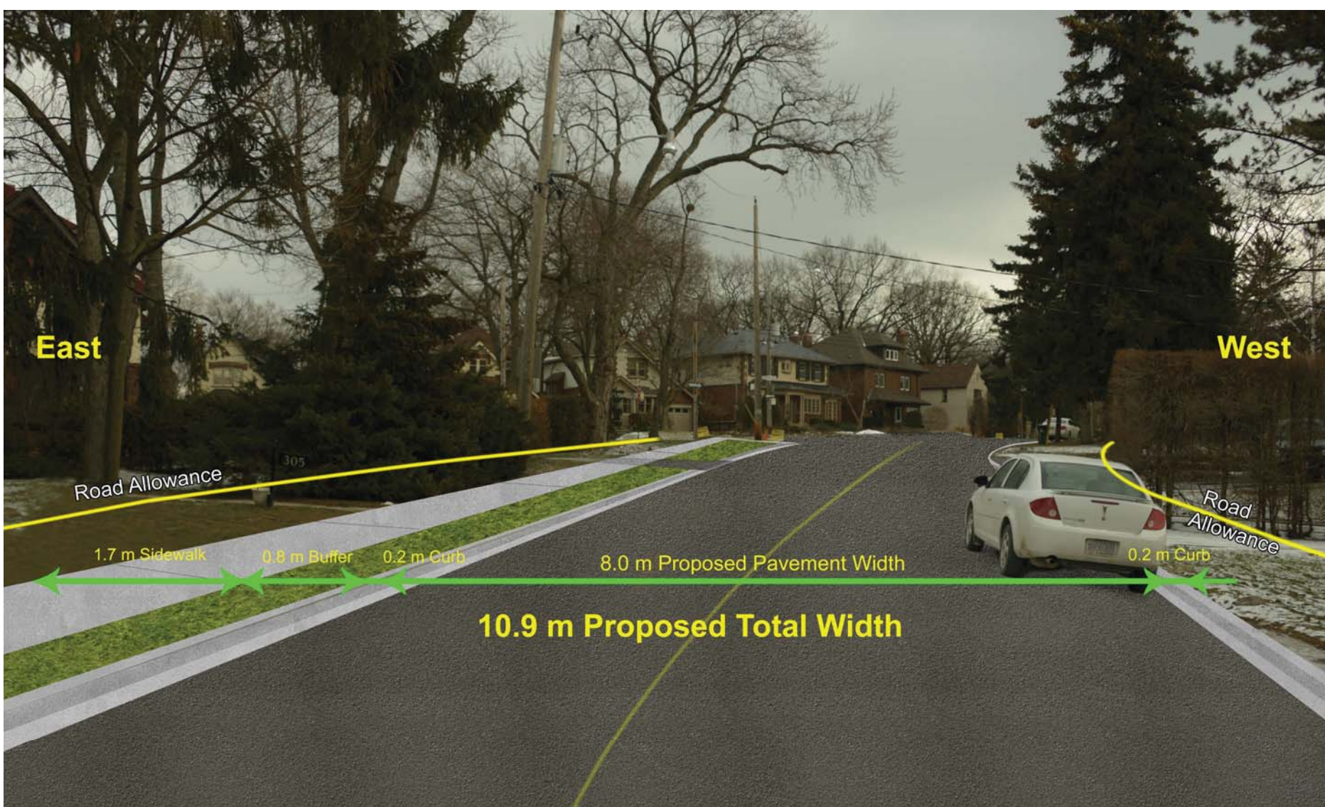
Proposed Road Cross Section
