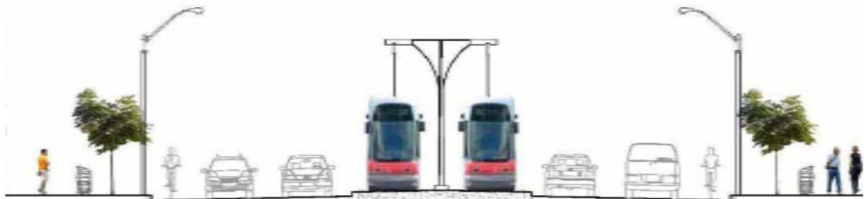
Figure 1-3 Finch LRT Typical Midblock Cross Section (Source: Etobicoke-Finch LRT TPAP, 2010)
