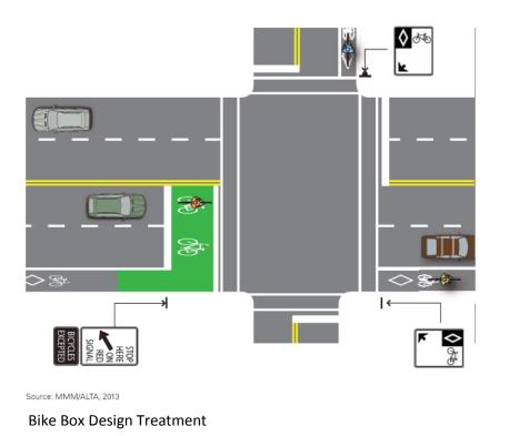
Figure 2: Intersection Design Examples.<sup>180</sup>
