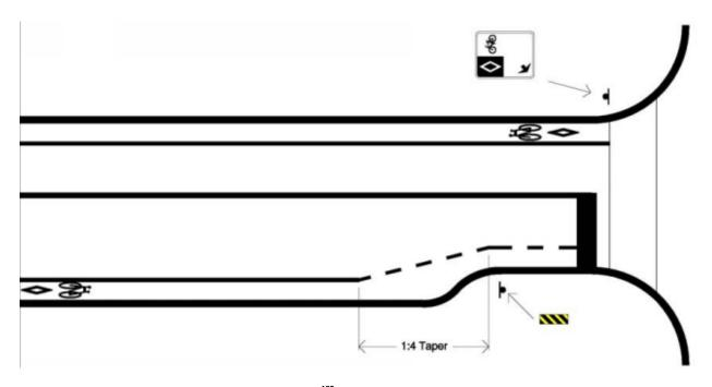
Figure 10: Bike Lane Tapered at Intersection with Curb Extension.<sup>182</sup>
