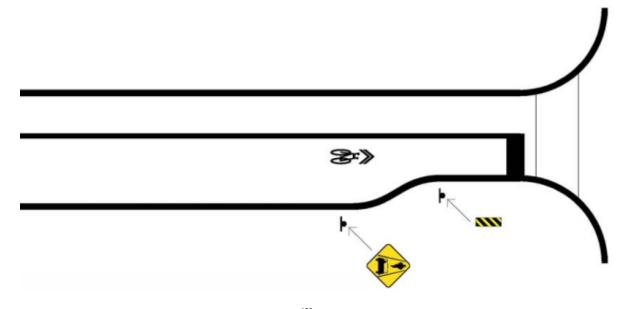
Figure 9: Sharrow Application at Intersection with Curb Extension.<sup>182</sup>
