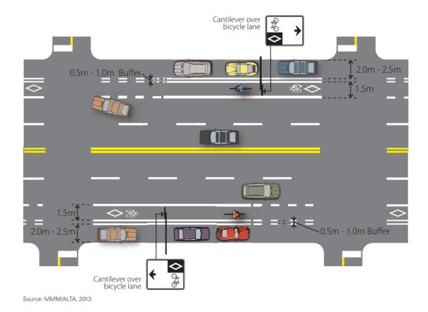
Figure 8: Bicycle Lane on Two-Lane Two-Way Road with On-Street Parking.<sup>180</sup>
