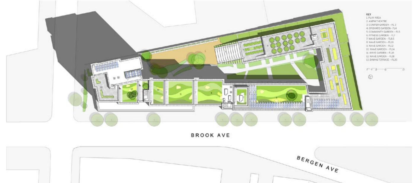
The 20-storey tower element at the corner terraces down to a lower base building which forms the courtyard. Rainwater makes its way down the terraces and is harvested by the green roofs. The community gardens on the wide side form a more structured outdoor area. The remainder of the greenspace is flexible to accommodate a variety of play.
