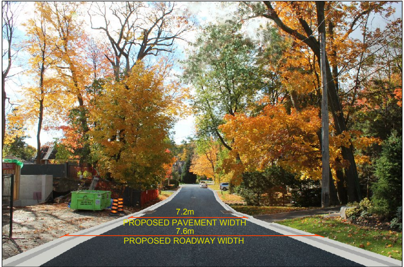
FIGURE F11 ILLUSTRATION OF EXISTING AND PROPOSED ROAD DIMENSIONS - FIDELIA AVE
