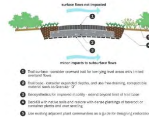
Typical Trail Construction in Wet Soils
