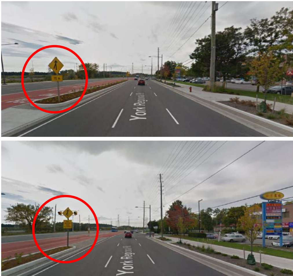
Figure 5-3: Signage Allowing the Merging of Exclusive Transit Lane with General Purpose Lane (GPL)
