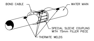
PIPE JOINT BONDING SLEEVE COUPLING BONDING
