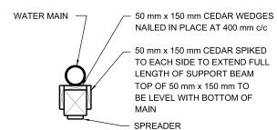
ALL VOIDS BETWEEN SUPPORT BEAM AND MAIN ARE TO BE FILLED WITH EXCAVATED MATERIIAL AND THROUGHLY COMPACTED
