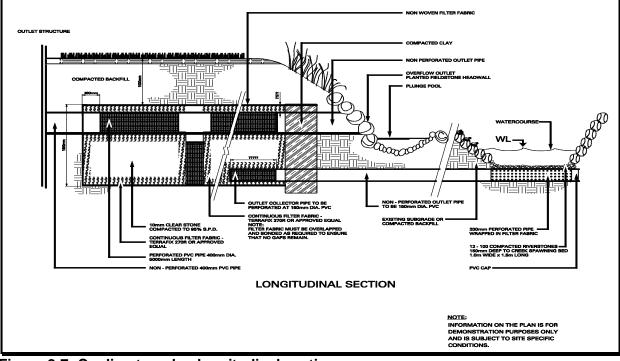
of the trench. It is preferred that the cooling trenches have multiple outlets in order to simulate the natural pattern of discharge to the downstream watercourse as seen in Figure 2-7 and 2-8.
