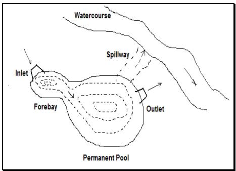
Figure 2-3: A typical stormwater management pond
