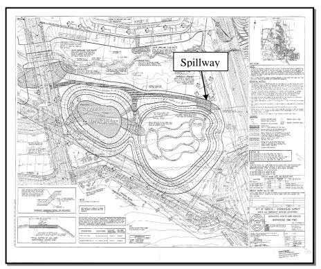
Figure 2-13: Spillway design at Morningside stormwater management pond
