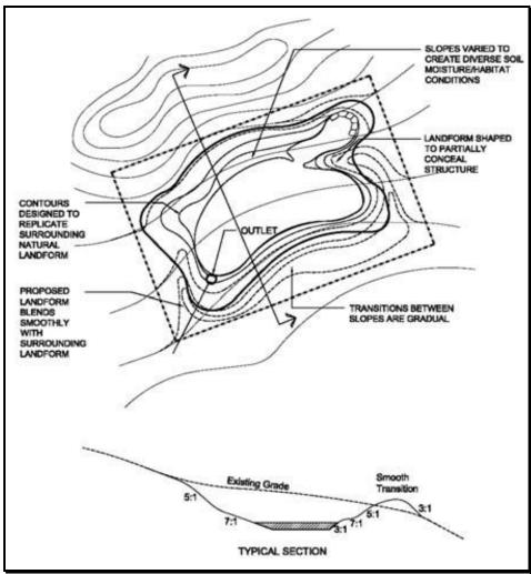
Figure 2-1: Landform Grading – Recommended Design <sup>1</sup>
