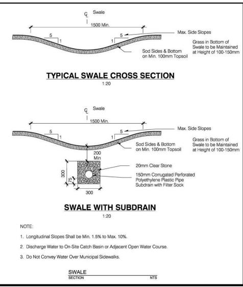
Figure 2-10: Typical swale cross section
