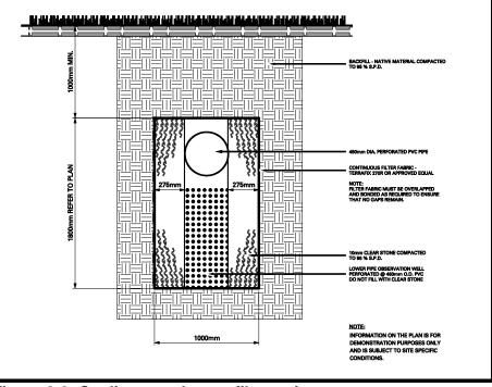
Figure 2-8: Cooling trench – profile section
