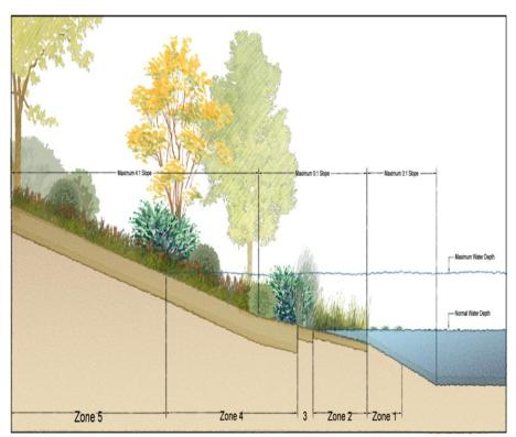
Figure 2-4: Five landscaping zones for typical stormwater management pond (wet pond)
