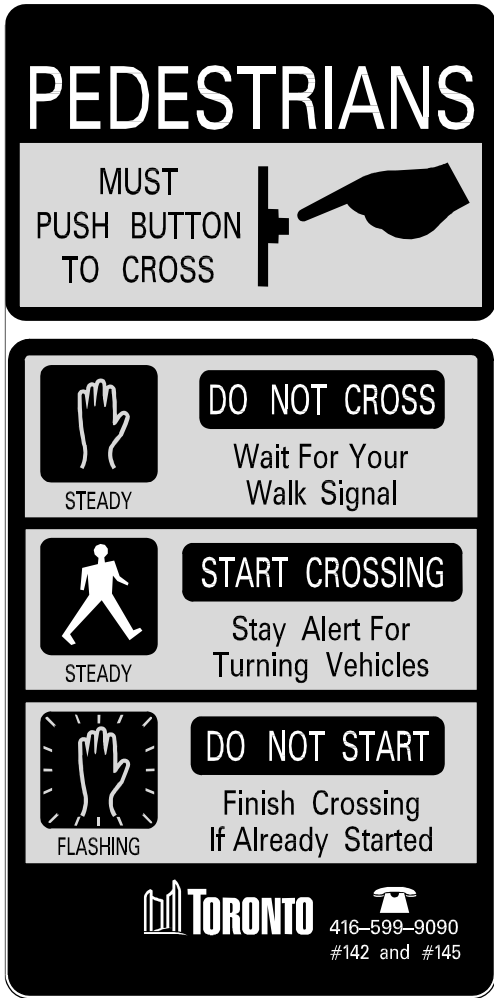
TYPE A: (M-6005) SEMI-ACTUATED /HELPING HAND DISPLAY (405 mm x 200 mm)
