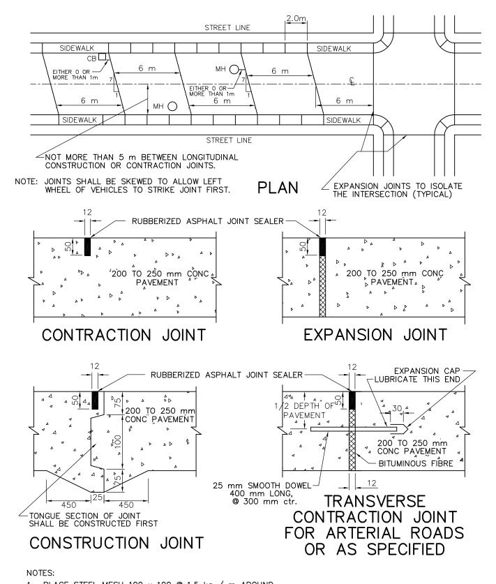
PLACE STEEL MESH 100 x 100 @ 1.5 kg / m AROUND MANHOLES AND CATCH BASINS TO COVER AREA ENCLOSED BY 1.5 m FROM THE APPURTENANCE, AND BE CLEAR OF JOINTS BY 150 mm.
