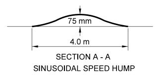
USED TO ACHIEVE A DESIRED SPEED OF 30 km/h
