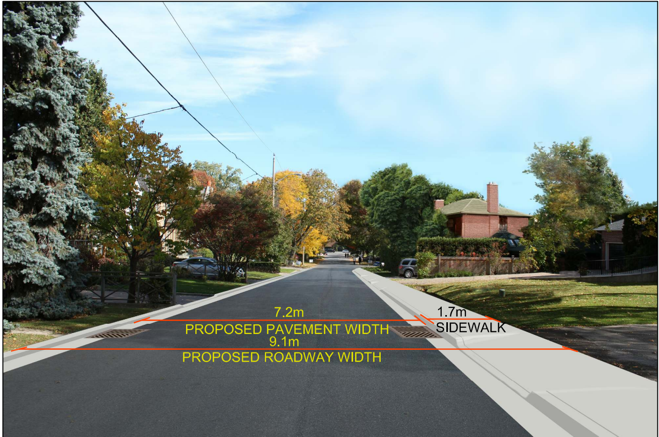
FIGURE DL1 ILLUSTRATION OF EXISTING AND PROPOSED ROAD DIMENSIONS - DAWLISH AVENUE
