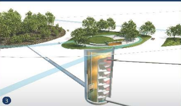
3 A Baffle Drop Structure will be used to convey flow from the existing Coxwell Sanitary Trunk Sewer into the new bypass tunnel.
