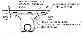
WHERE HOUSE CONNECTIONS OR CATCH BASIN LEADS CROSS A SEWER TRENCH, THEY WILL BE SUPPORTED ON A NEW 100 mm x 200 mm TIMBER WHICH HAS A MINIMUM BEARING OF 1000 mm AT EACH END, ON UNDISTURBED GROUND. CONNECTION MUST BE PROPERLY SHIMMED. SEE DETAIL ABOVE - OR BEDDED ON 15 MPa CONCRETE FILL, TO SPRINGLINE, AS PER DETAIL BELOW.
