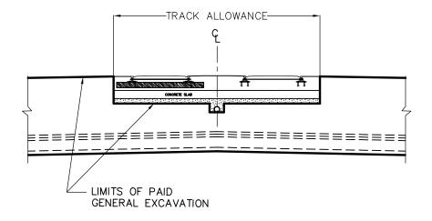
NOTE: IF EXISTING TRACK SYSTEM IS BURIED, ALL MATERIAL ABOVE THE TOP OF RAIL IS INCLUDED IN THE UNIT PRICE BID FOR GENERAL EXCAVATION.
