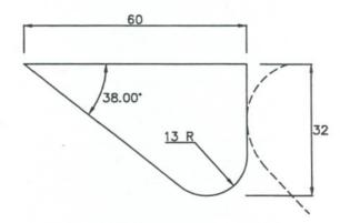
TEMPLATE FOR WOODEN FORM FOR A 49.60kg T RAIL GROOVE
