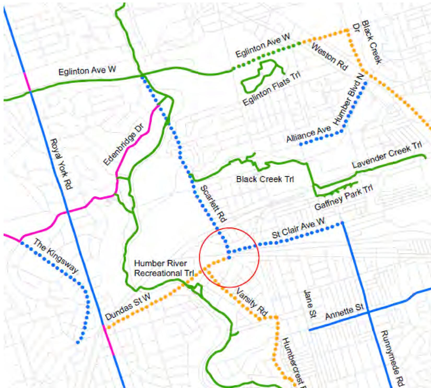
The City of Toronto is planning to install a physically separated cycle track under the Scarlett Road Bridge as part of the bridge reconstruction.
