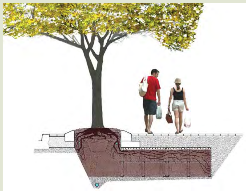
Figure 34. Soil cells being used to increase soil volumes for planting in a commercial area.
