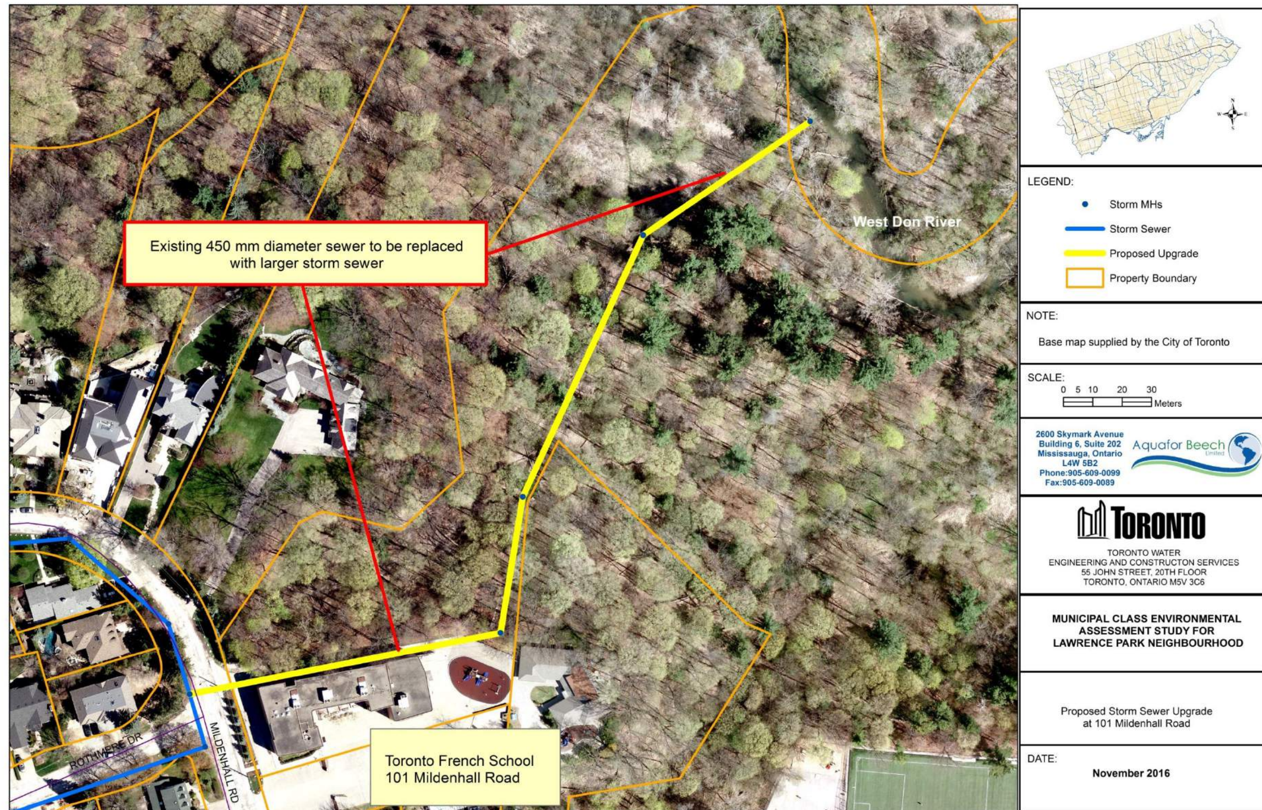
Figure 2.1: Proposed Storm Sewer Upgrades at Site 1
