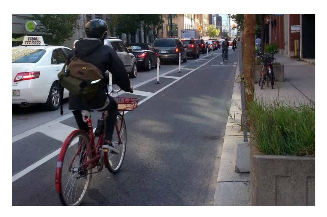
Cycle Track: Dedicated cycling facility that features separation elements, such as parked cars and flexi-posts, between the bike lane and the traffic lane, as well as between the bike lane and parked cars.
