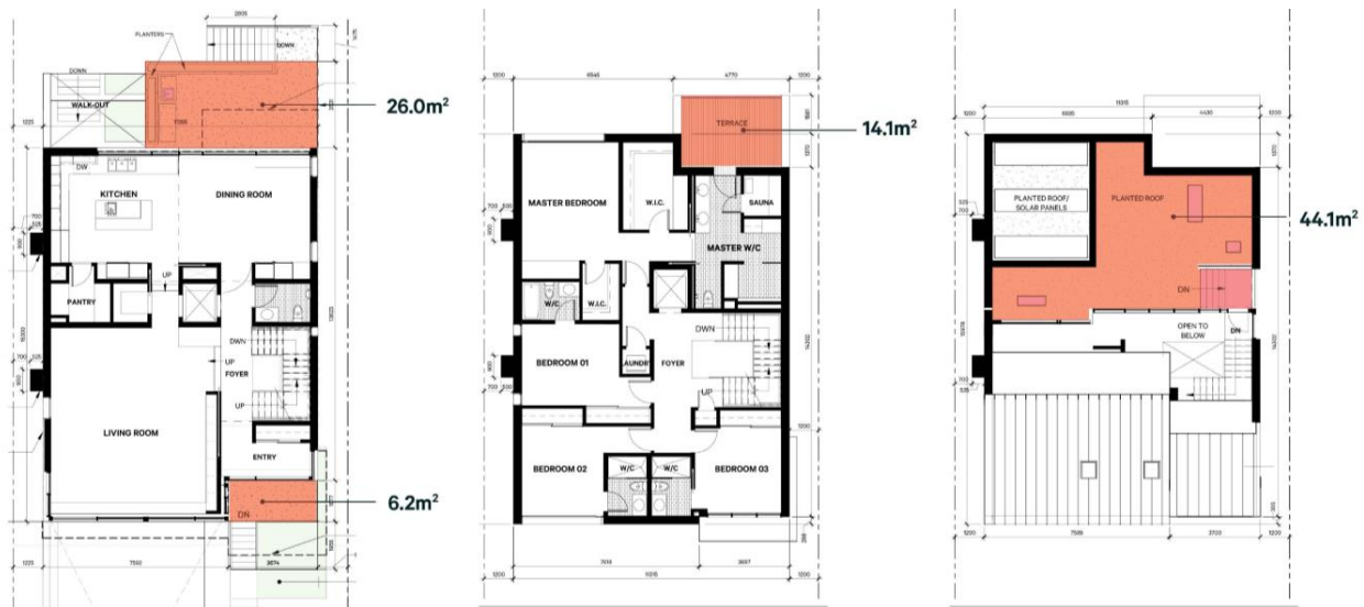
Figure 3. Balconies shaded; left to right: ground floor, third floor, green roof
