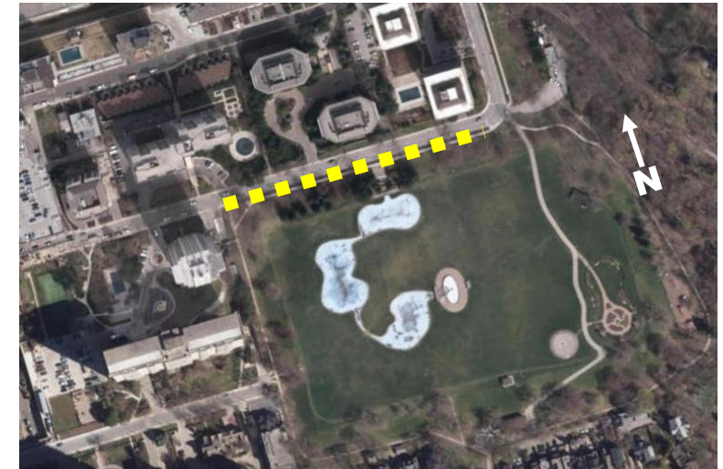
Rosehill Avenue Temporary Sidewalk will be installed with protective barriers (yellow dash)
