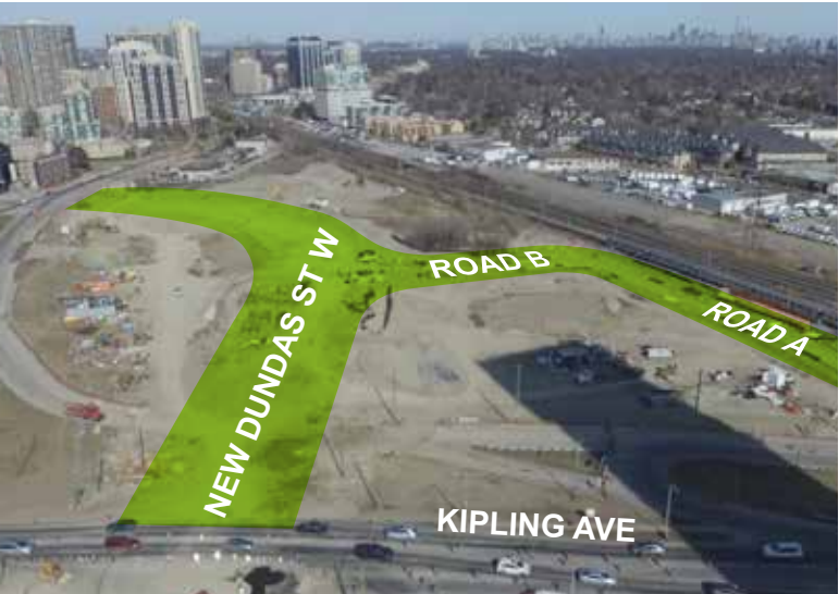
The new Dundas Street West alignment and Roads A and B are being constructed, including new water-mains, separate storm water and sanitary sewers, streetscaping (including landscaping, street lighting and underground utilities), road resurfacing and curb installation.
