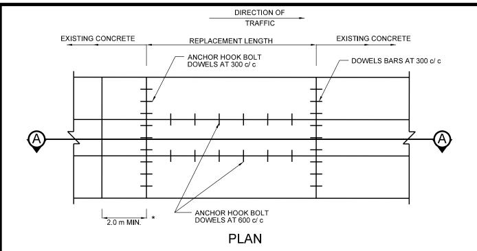
\* IF PROXIMITY OF FULL DEPTH REPAIR TO EXISTING JOINT OR CRACK IS 2.0 m OR LESS, EXTEND CONCRETE REPLACEMENT TO 300 mm BEYOND JOINT OR CRACK.
