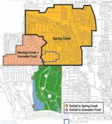
Stormwater Catchment Areas
