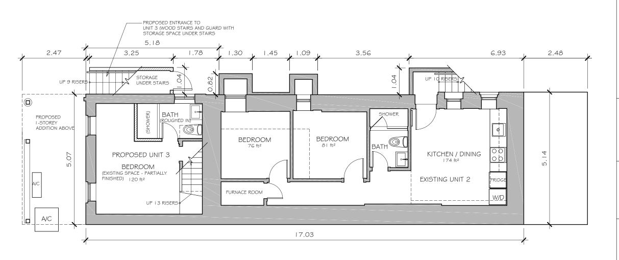
EXISTING REAR BASEMENT SPACE TO BE CONVERTED INTO BEDROOM AND BATHROOM FOR PROPOSED UNIT 3. FRONT BASEMENT SPACE IS EXISTING UNIT 2 -NO CHANGES PROPOSED TO THIS UNIT.
