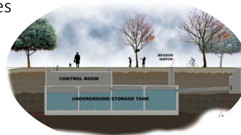
Example of underground storage tank design.
