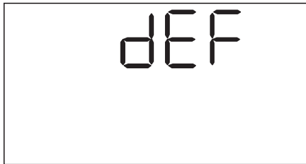
Figure 12. Restoring the Factory Defaults
