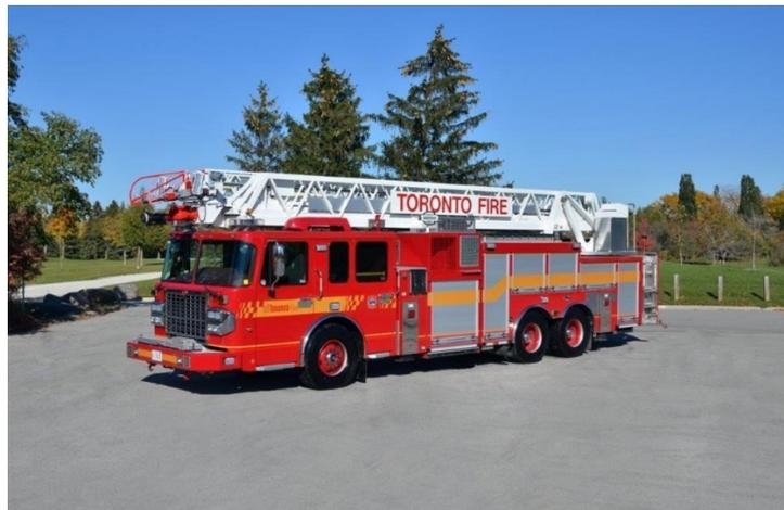
These ladders are capable of reaching several stories and allow firefighting personnel to position themselves in a raised position (Jon's Mid America, 2017). Ladder Trucks have the ladder fixed to the truck. Ladder sizes vary, with 75 foot and 105 foot ladders being common lengths.<sup>18</sup> The NFPA Standard 1901 requires that aerial ladders have a minimum vertical height of 50 feet (15m) (NFPA, 2016, Chapter 19, Section 19.2.2). Trucks with water towers must
