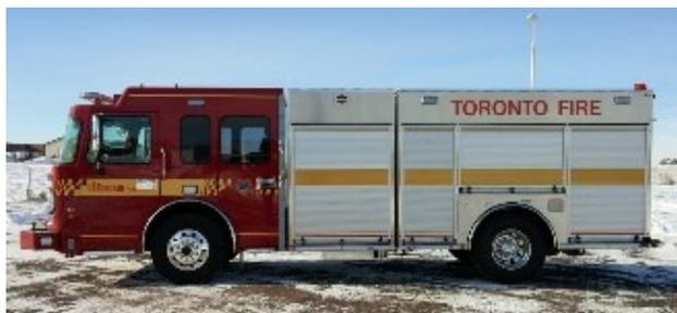
Tankers, Tanker Trucks, Foam Tenders, and Water Tenders are designed to transport or pump large amounts of water wherever it is needed. Tankers come in many different sizes. They are generally used in rural locations where pressurized water is rarely readily accessible (Heavy Duty Direct, 2017a). Like other fire trucks, tankers carry firefighting equipment, such as hoses, nozzles, safety and rescue equipment, and hand tools (CFA, 2018).
