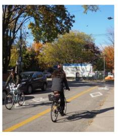
Contra-flow Bike Lane: allows cyclists to travel in two directions on a one-way street. Cyclists travel in one direction in the designated bicycle lane. When travelling in the opposite direction, the cyclist will travel in the shared lane.
