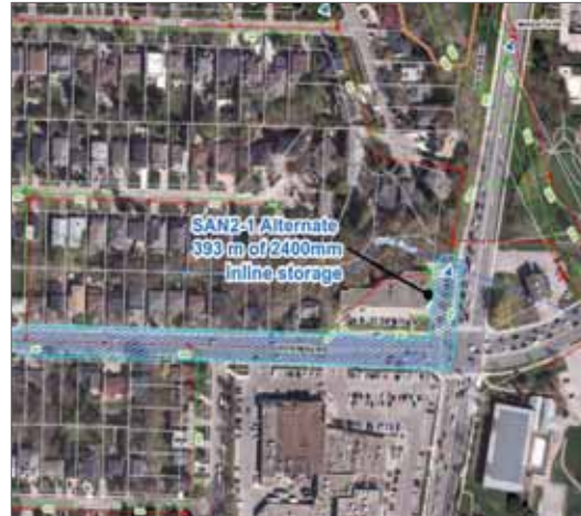
Alternative with works in ROW – 393 m of 2400mm inline Storage on Bayview Ave.
