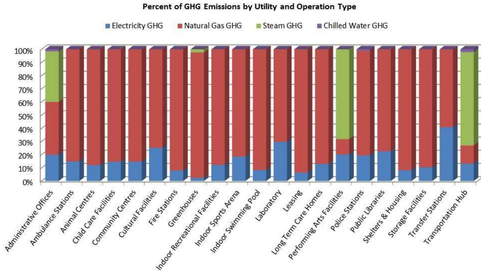
**Figure 7: Building Greenhouse Gas Distribution by Operation Type**
