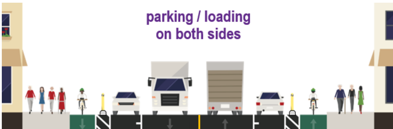
Example of proposed street configuration for wider sections: bike lane with on-street parking on both sides
