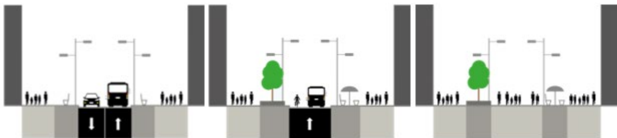
Figure 2: The three street design options: Option 1 (Two-Way Traffic), Option 2 (One-Way Traffic), Option 3 (Pedestrian Priority Zone).
