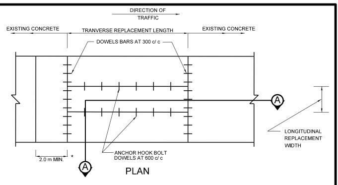
\* IF PROXIMITY OF FULL DEPTH REPAIR TO EXISTING JOINT OR CRACK IS 2.0 m OR LESS, EXTEND CONCRETE REPLACEMENT TO 300 mm BEYOND JOINT OR CRACK.
