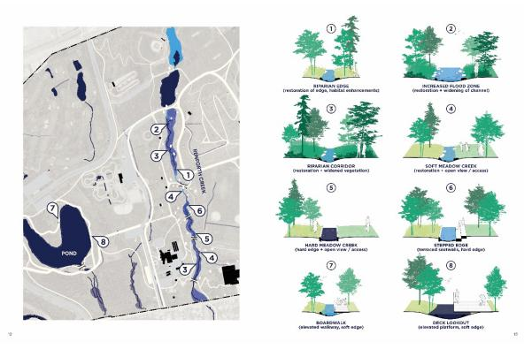
The diagram above shows the possible types of edges along Renforth Creek and the pond. The edge types are illustrated on the right and are coded on a close up map on the right.
