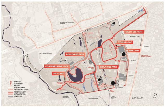
The diagram above shows the proposed circulation network for the park. The use (multi-use, pedestrian, designated bike) is shown in the legend to the bottom left.
