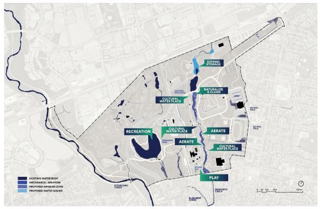
The diagram above proposes possible relationships to the water edges. It also proposes locations for new storage for stormwater management, and areas where waterways could be naturalized in order to clean the water and provide better habitat. We have also proposed two ponds for aeration to aid with water flow. Locations marked as "cultural water place" are proposed for improved access and views to the water.
