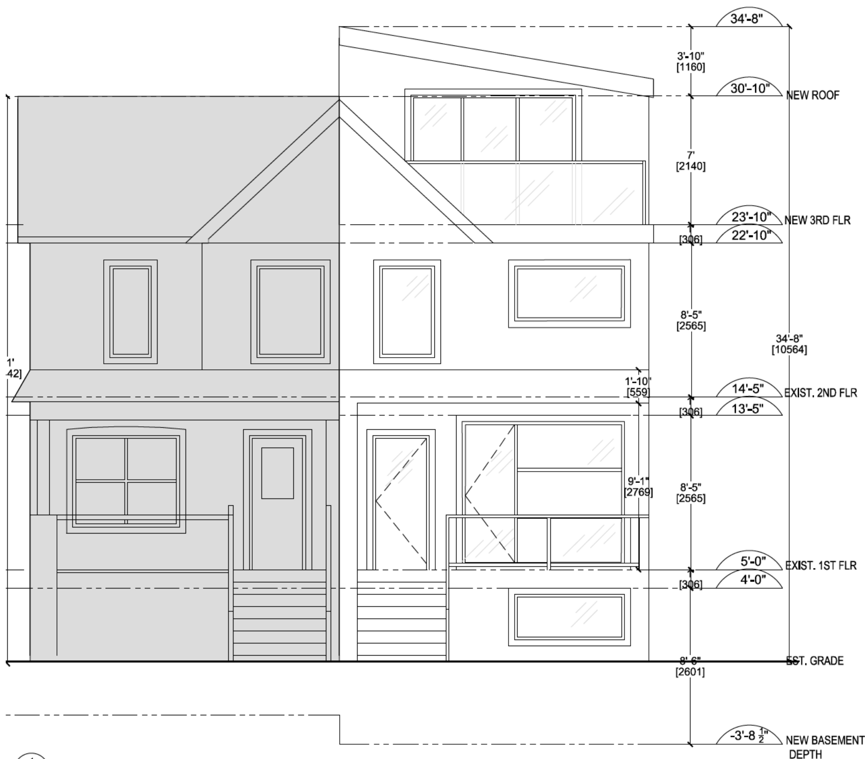
1 A3.5 PROPOSED WEST ELEVATION (FRONT) 3/16" = 1'-0"
