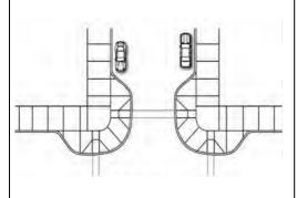
Curb extensions, also known as bump-outs, reduce the pavement width at intersections by extending the curb into the roadway.
