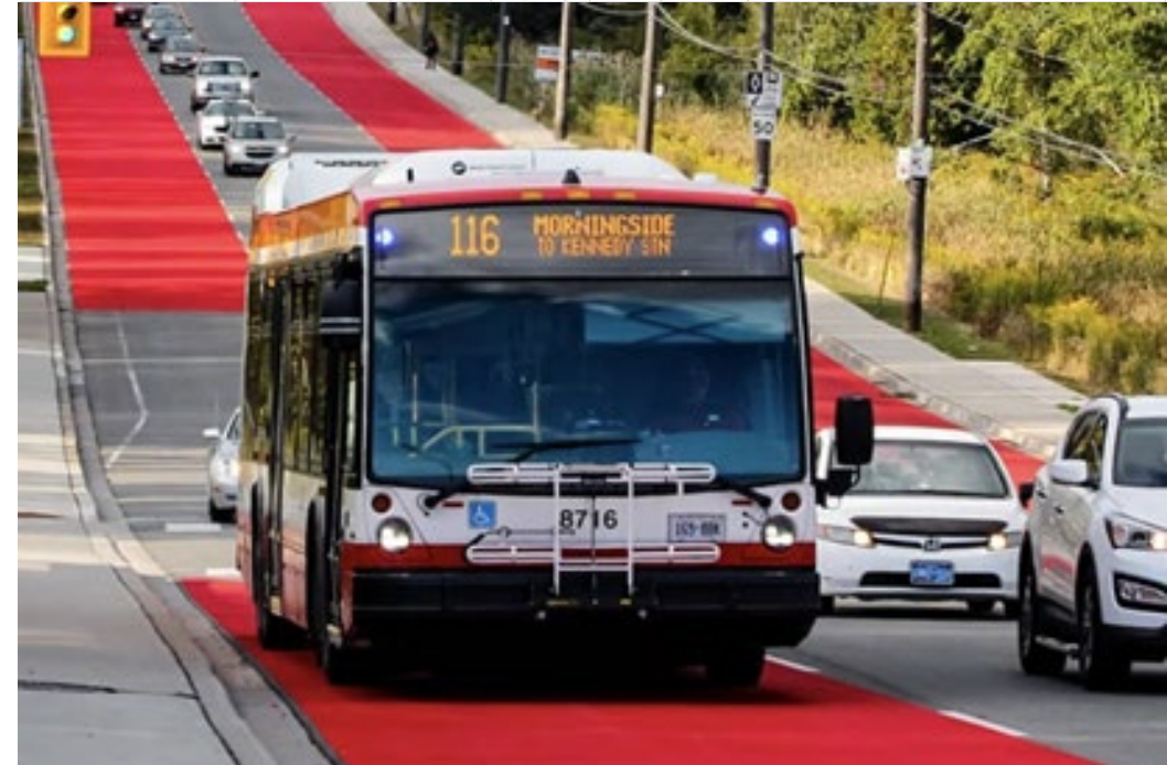
RapidTO: Priority Bus Lanes are identified using red surface paint.
