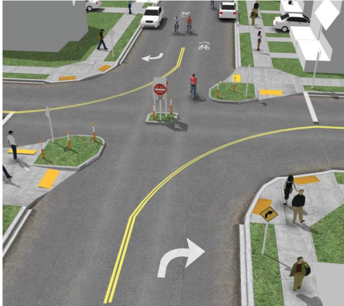
Diagonal diverters: vehicles must turn; bikes and pedestrians allowed through
