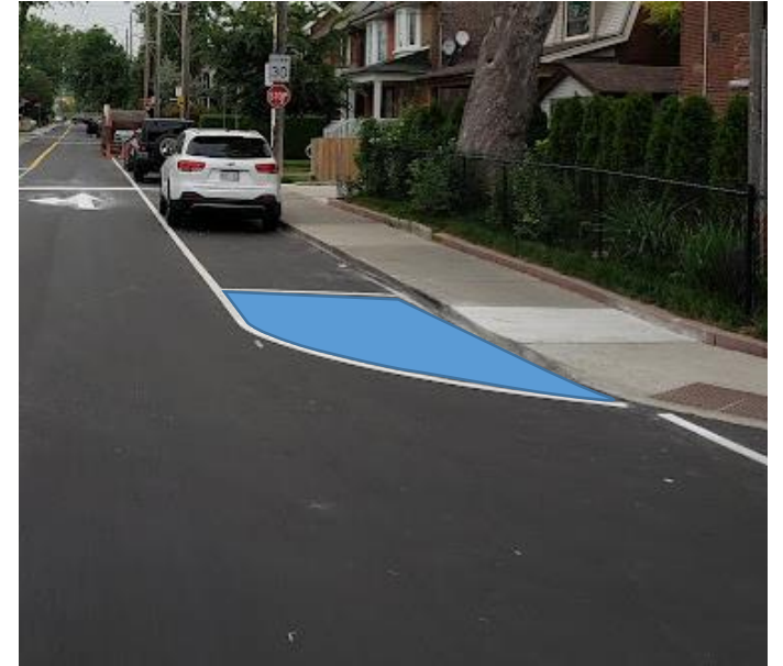
Parking set back from the corners to allow for better sight lines and for trucks to turn
