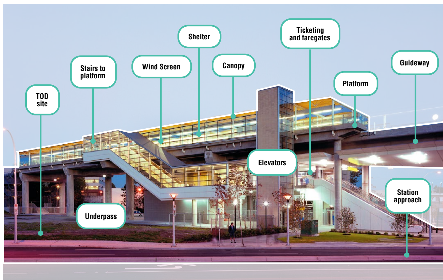
Figure 2: Diagram depicting the various components of a typical elevated station, Gilmore SkyTrain Station (Photo Credit: Perkins&Will)
