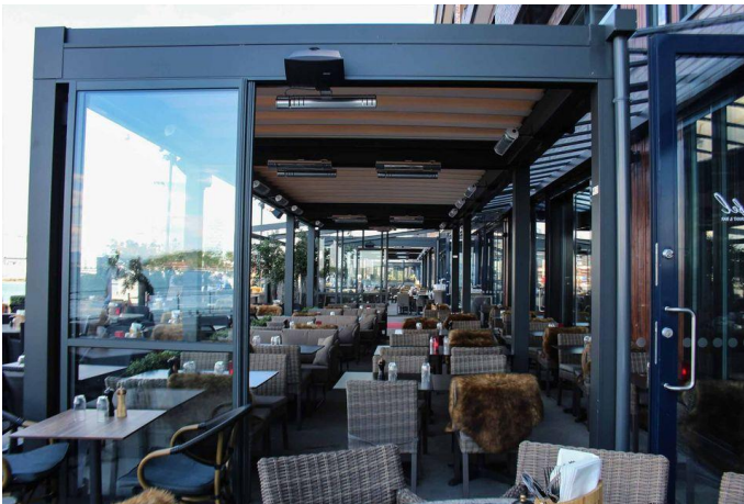
Sorenga, Oslo: Permanent patio structure with sliding windows to allow for changes in weather for different seasons and built in heating units
