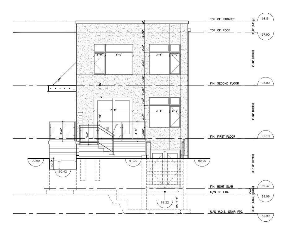
PROPOSED REAR (WEST) ELEVATION
