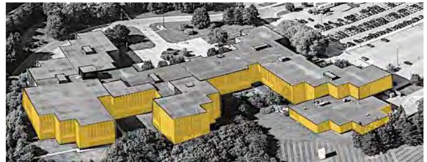
*b) 1150 Eglinton Ave. Proposed retention of Brick Masonry wall (in Orange)*
