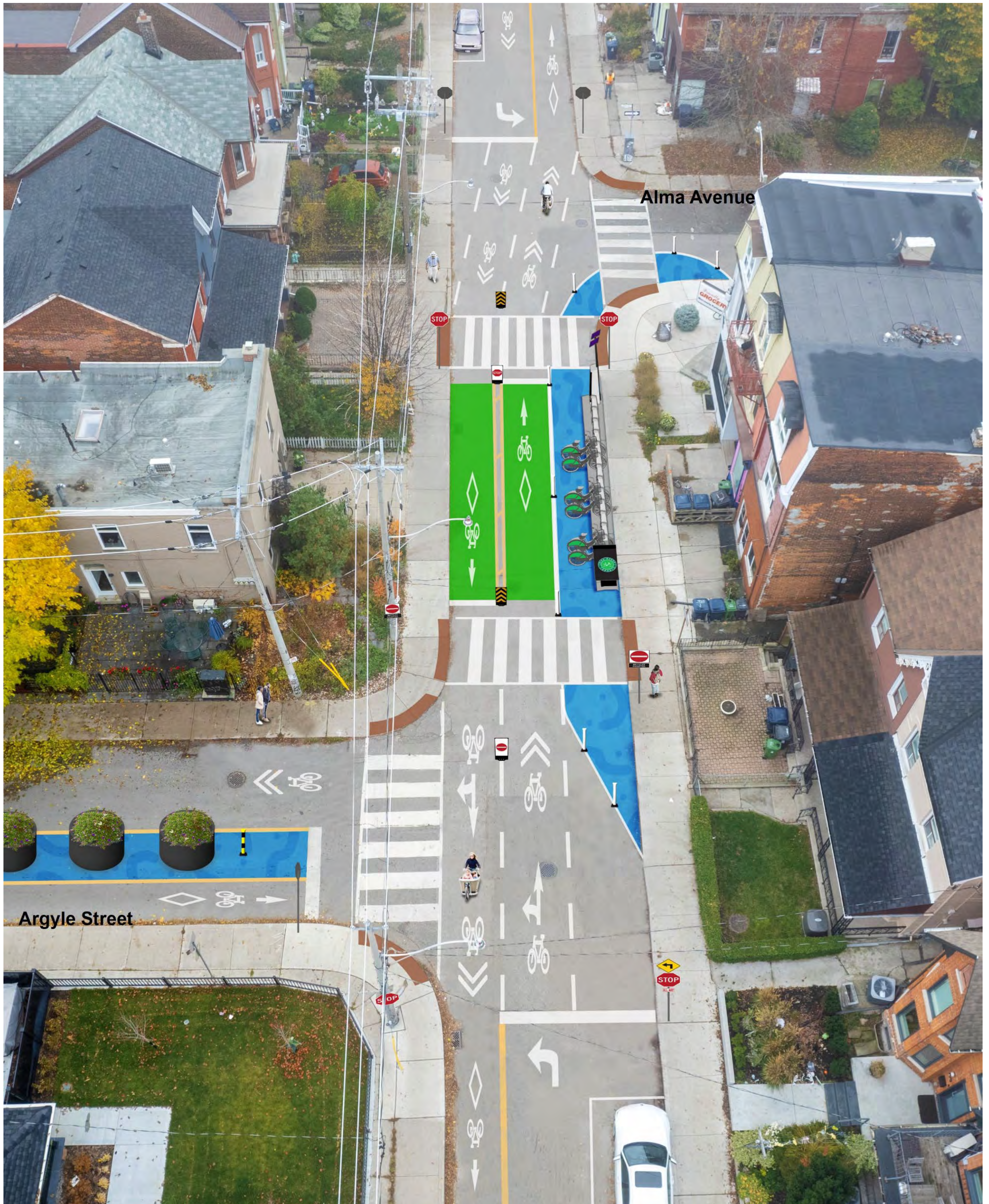
Artistic rendering of the cycling-only block between Argyle Street and Alma Avenue
