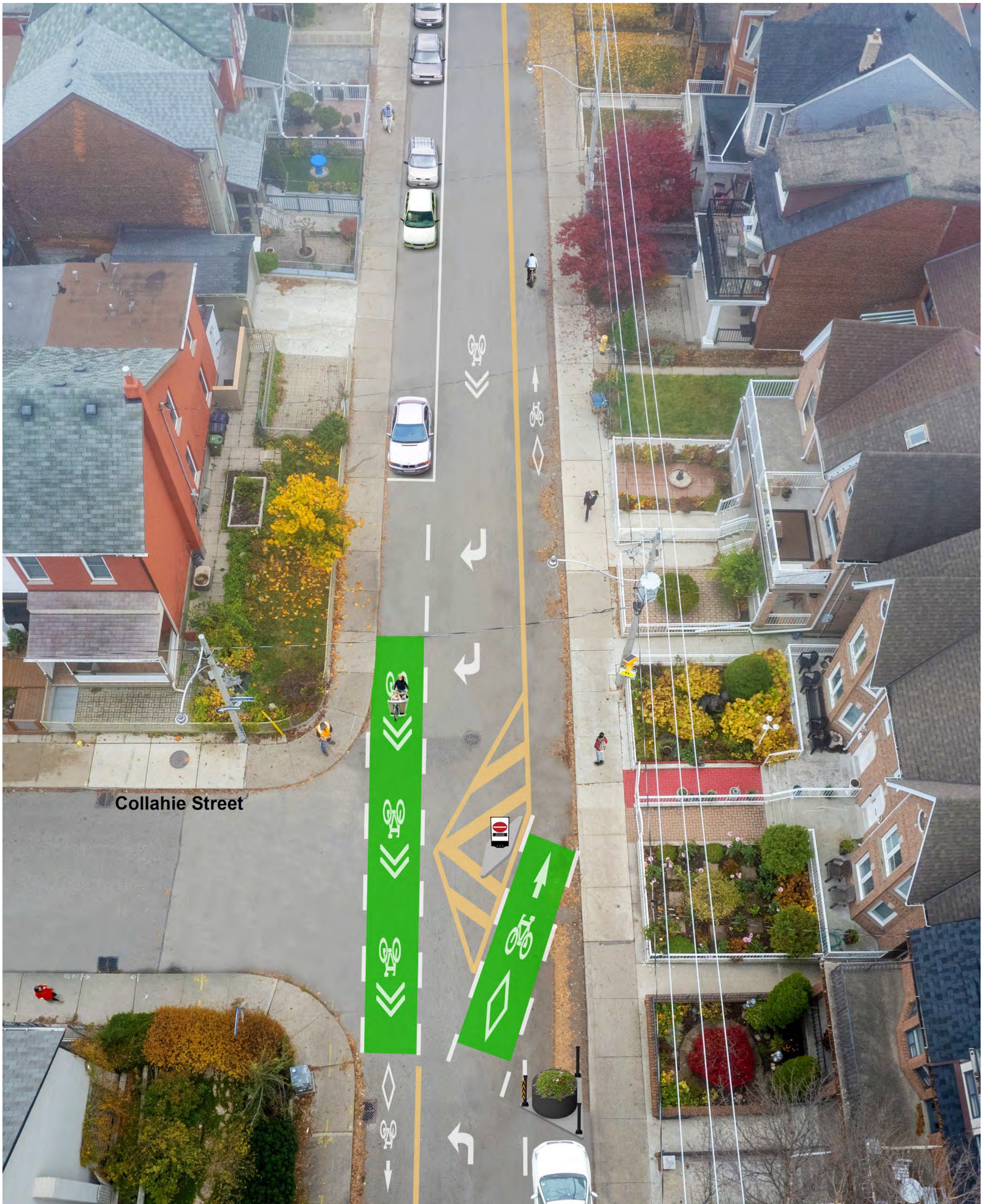
Artistic rendering of the proposed direction change on Gladstone Avenue at Collahie Street
