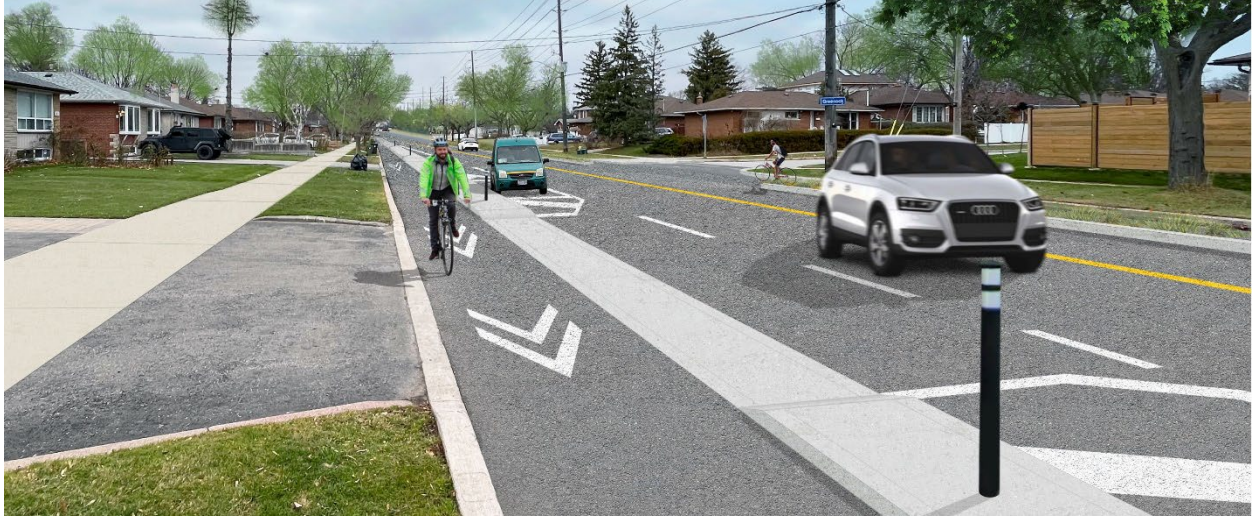
Rendering of proposed addition of protected one-way cycle track to Scarborough Golf Club Road
