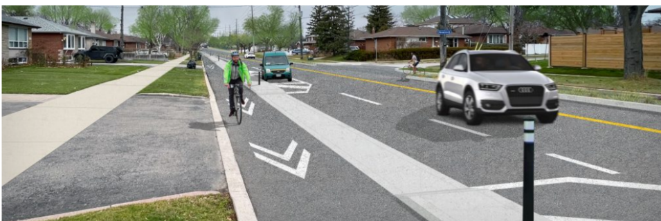
An artist's rendering of proposed addition of protected one-way cycle track to Scarborough Golf Club Road
