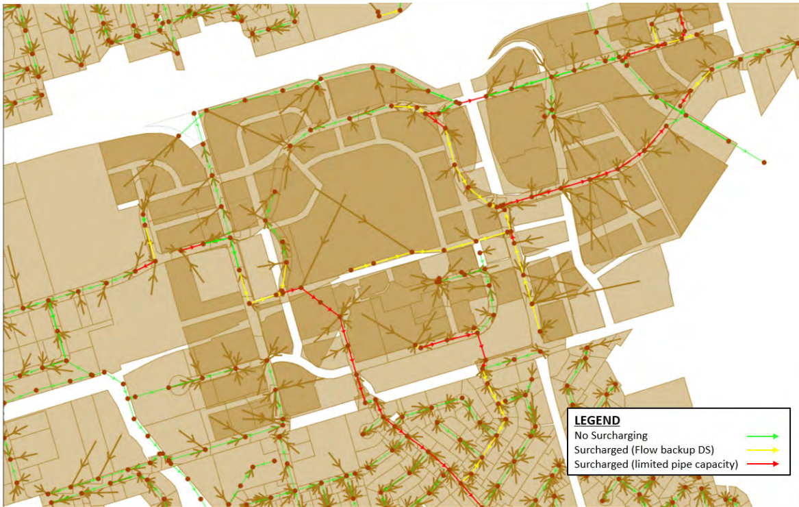
Figure 12.6 Existing Pipe Network with Projected Wastewater Loads
